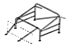
Side View-Low Front Bar Forward Bracing
