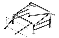
Side View-Low Front Bar Forward Bracing
