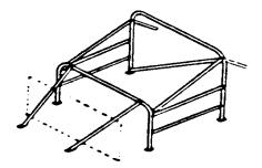
Side View-Low Front Bar Forward Bracing
