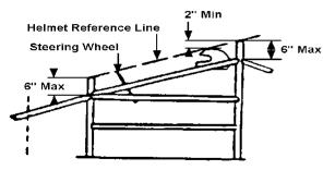
Side View-Low Front Bar Forward Bracing
