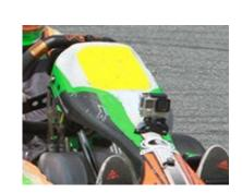
The mounting position on the **steering column fairing**/front panel is fixed horizontally, in the middle axis, and a minimum 10 cm below the bottom edge of the number area of the panel. The camera should not block the view of the number from the front.
