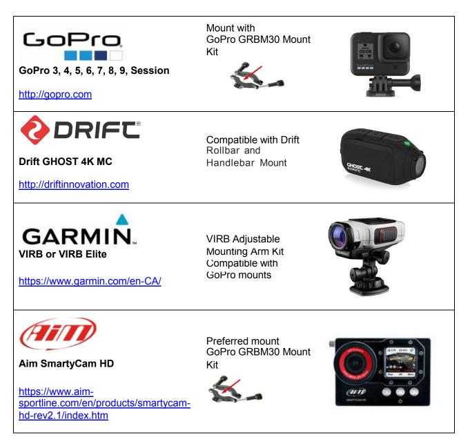
Two cameras can be mounted on a kart at any time.
