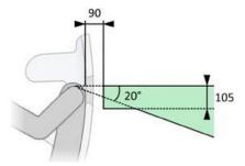
6.5.2 The shoulder strap anchorage points must be symmetrical about the vertical and longitudinal plane passing through the centerline of the seat. When viewed from above, the angle between the straps must not be out of the 10°-25° range and it is recommended it is approximately 20°-25°.
